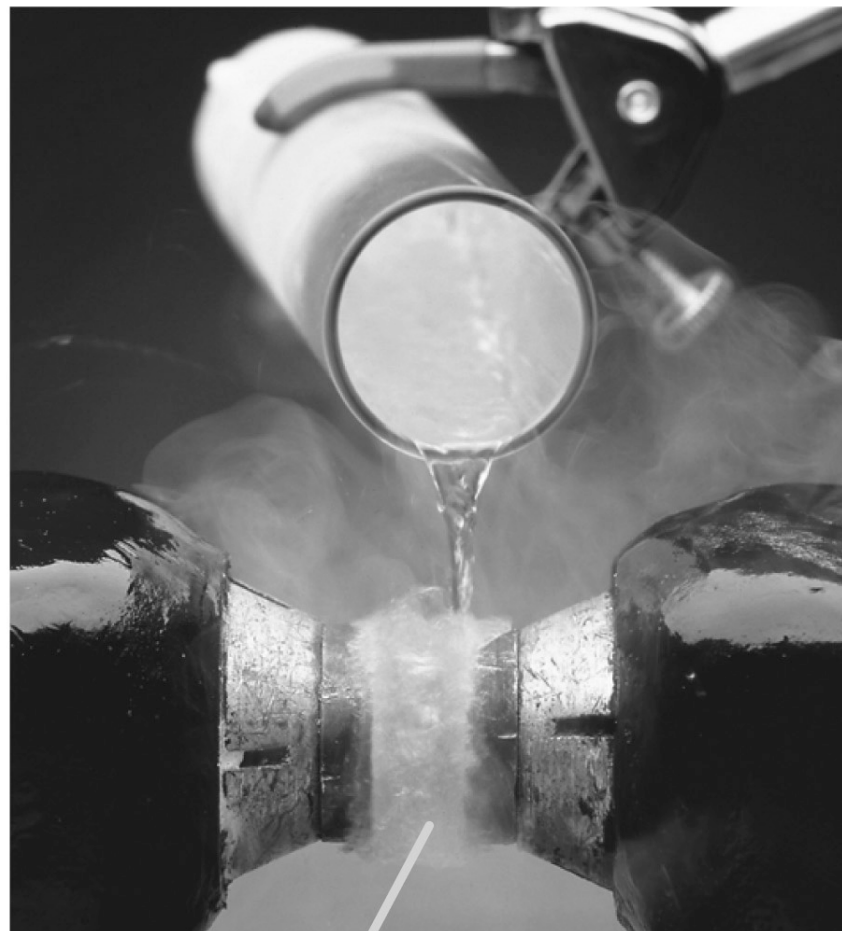
Liquid oxygen is paramagnetic and is held between the poles of the magnet.
